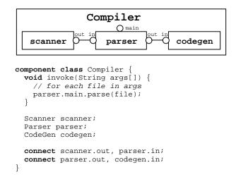
Figure 2. A graphical compiler architecture and its ArchJava representation. The Compiler component class contains three subcomponents—a Scanner, Parser, and CodeGen. This compiler architecture follows the well-known pipeline compiler design [GS93]. The scanner, parser, and codegen components are connected in a linear sequence, with the out port of one component connected to the in port of the next component
